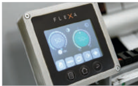
Automatic vertical alignment control panel
